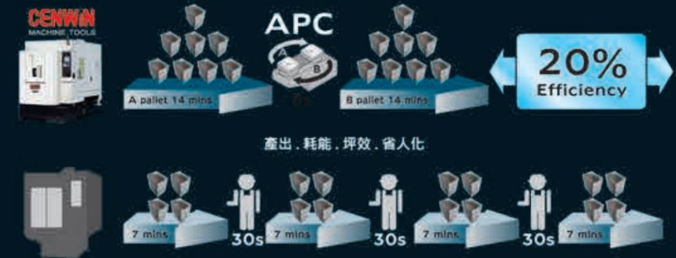
Cenwin H-4035 is equipped with 2 Automatic Pallet Changer (2APC) which changing time only takes 8 seconds to meet higher efficiency.
