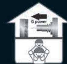
Cenwin H-4035 brings horizontal G-force is able to moderate the vibration impact on floor effectively.
